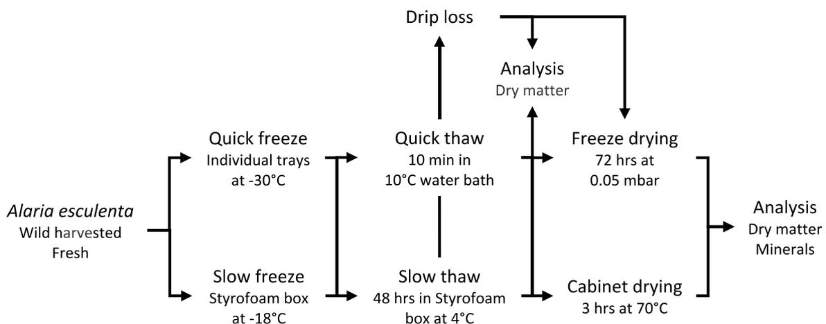
**Fig. 2** Process flow chart for supplemental experiment: Quick and slow freezing and thawing of *Alaria esculenta*
